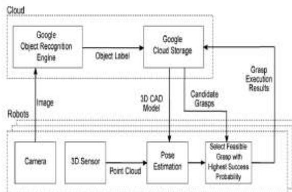
Figure.1. System Architecture for Cloud-based object recognition for grasping
