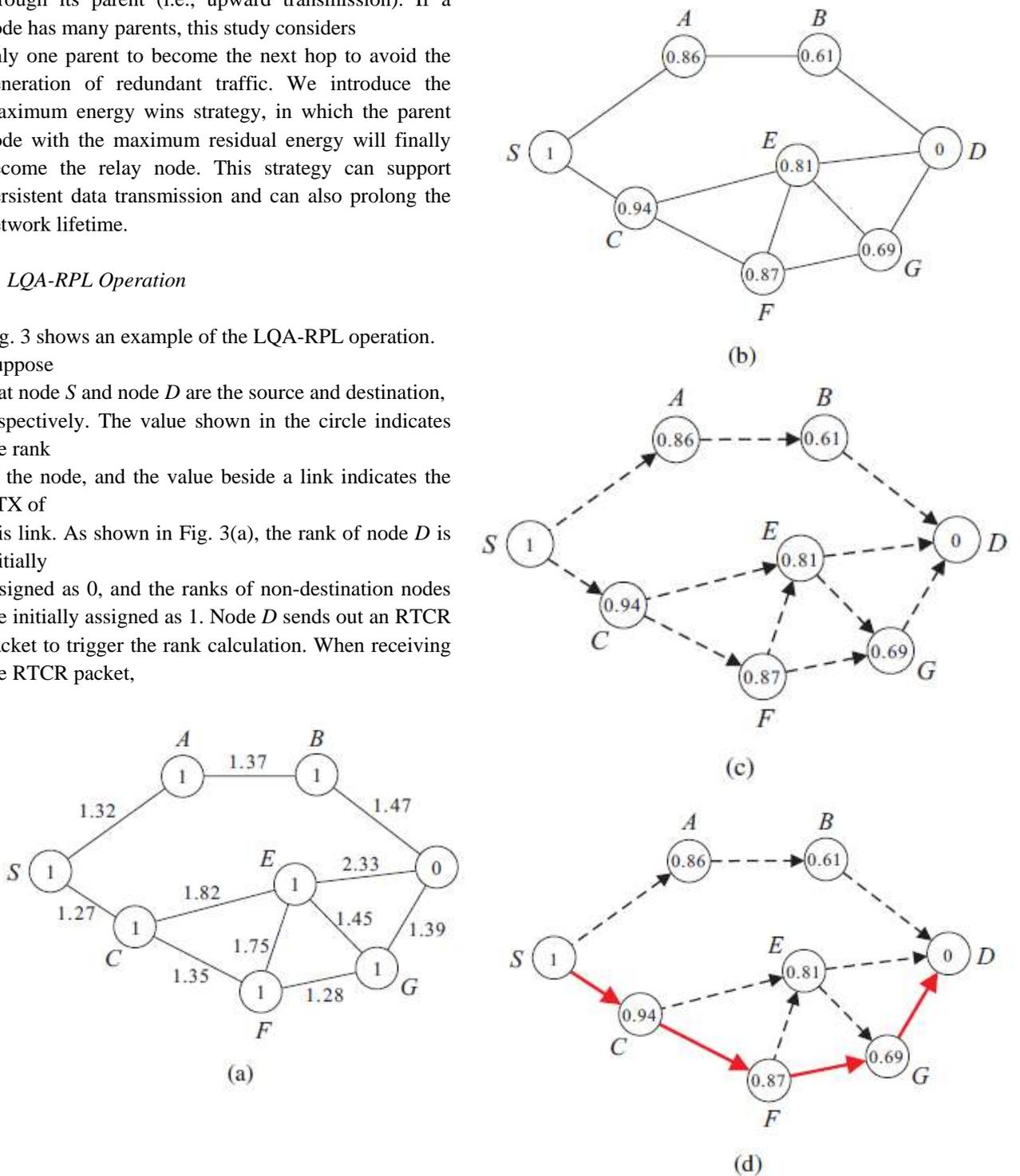
Fig. 3. Example of the operation of LQA-RPL. (a)Assignment of the initial rank of each node. (b) Result of rank calculation. (c) Result of DODAG construction. (d) Result of path determination. Suppose  $E_C^{res} > E_A^{res}, E_F^{res} > E_E^{res}, E_G^{res} > E_E^{res}$  where  $E_i^{res}$  is the residual energy of node *i*.
