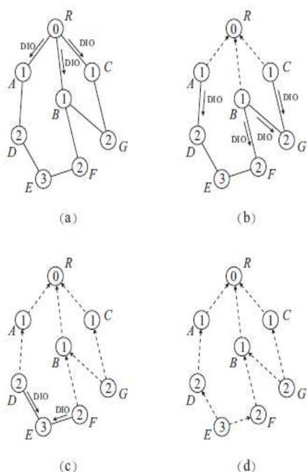
Fig.1. Example of the DODAG construction. The value at each node indicates the rank of this node. (a) The root broadcasts a DIO message to trigger the DODAG construction. (b) Nodes  $A$ ,  $B$ , and  $C$  have determined their own parents. (c) Nodes  $D$ ,  $F$ , and  $G$  have determined their own parents. (d) Node  $E$  has determined its parents, and finally the DODAG is constructed
