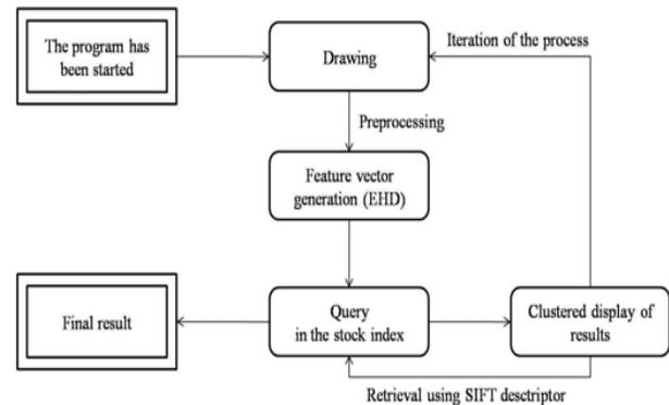
Fig. 4. The data flow model of the system from the user's point of view
