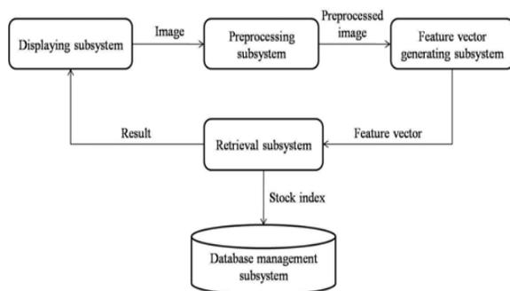
Fig. 3. The global structure of the proposed system.
