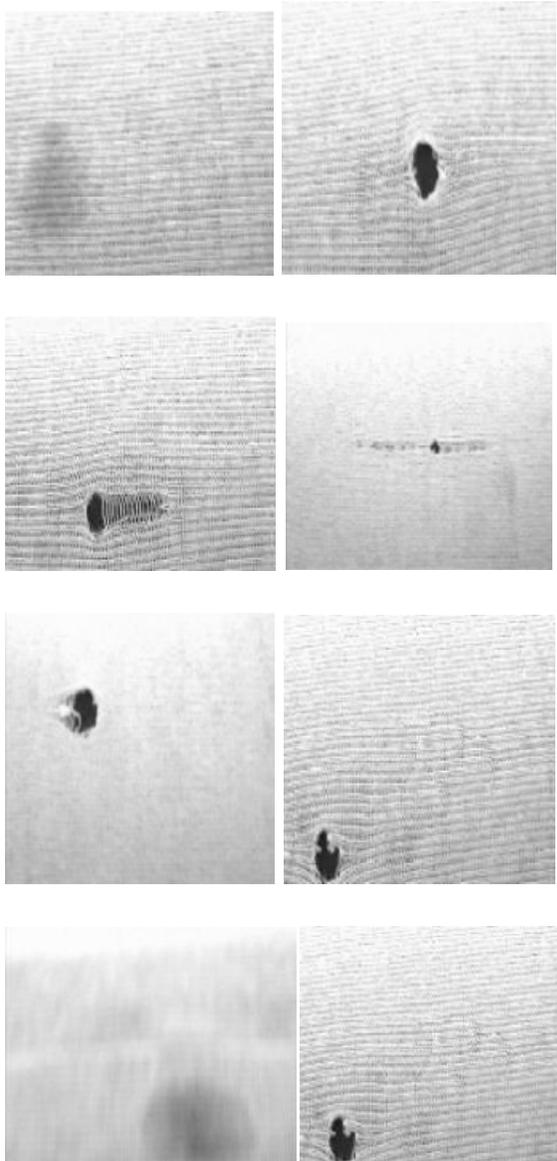
Fig: An image of a fabric with different defects
