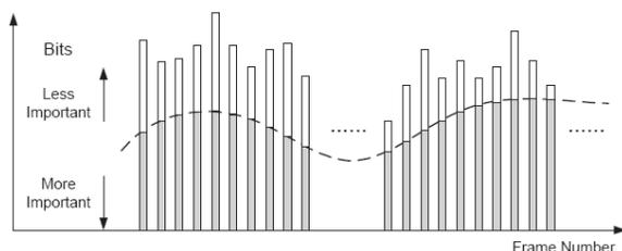
**Figure 2: Bit stream scaling in rate scalable video communications.**
