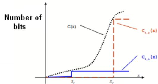
**Figure 4: A sample embedding function of FZDH in 1D.  $C_i$  is a reconstruction point of the quantizer.**
