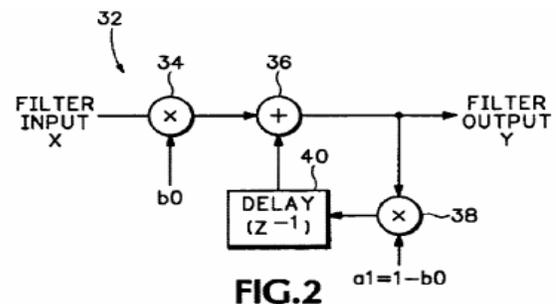
Figure 6: Adaptive Integrator process.
