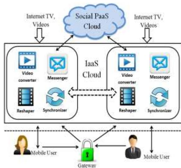
Figure 1: Architecture of Cloud MOV
