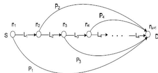
Figure: The major route consists of  $L_1, L_2, \dots, L_k$ . Each node in the primary route  $n_i$ , has an alternate path  $P_i$  to the destination. Alternate routes in [18].
