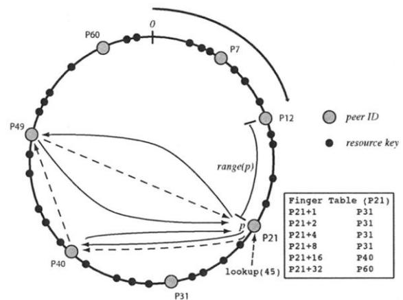
Fig. 3.1-Basic Chord operations.  $m$  is set to 6.
