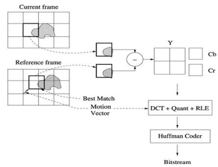
**Figure 3: Coding of P-frame.**
