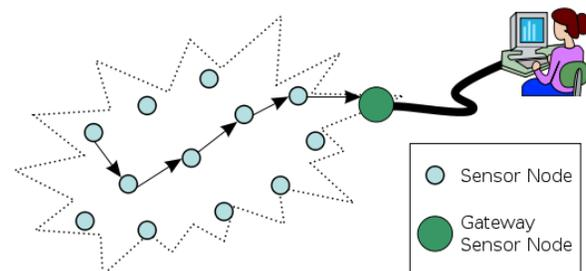
**Figure 1:** *Wireless sensor network with gateway interface.*
