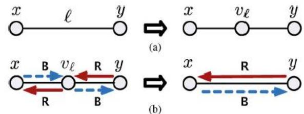
Figure: The construction of node-independent DAGs using a virtual node. (a) Expansion with virtual node. (b) Contraction to remove virtual node.
