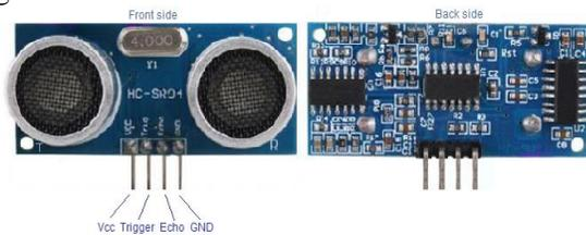
Fig 5: ultrasonic sensor
